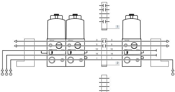
Pressure zone separation in ducts
