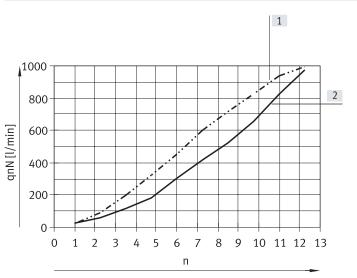
Standard nominal flow rate qnN as a function of the turns n of the regulating screw VABF-S1-1-F1B1-C
